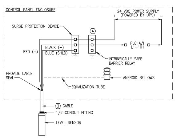
LEVEL SENSOR – WET WELL  $\langle 1 \rangle \langle 2 \rangle$  (4-20 Ma)
