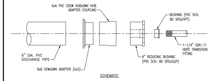
NOTE: THIS DETAIL REPRESENTS A DISCHARGE CONNECTION FROM A 1-1/4" LPS PIPE TO A 6" DIAMETER GRAVITY SEWER MAIN OR LATERAL. FOR DISCHARGE CONFIGURATION WITH PIPE SIZES THAT VARY FROM THOSE SHOWN ABOVE, APPROPRIATELY SIZED FITTINGS/ADAPTERS SHALL BE INCORPORATED.
