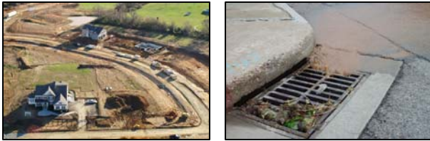
Figure 3. Development creates impervious surfaces that increase stormwater runoff, which carries nutrients, sediment, and other pollutants to waters.
