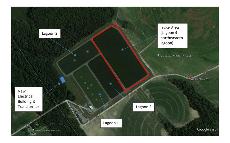
The lagoon is about 12 feet deep normally and the depth can fluctuate very slowly seasonally between 4 and 20 feet deep. The lagoon has a clay lined bottom which must not be penetrated or damaged by any anchoring system.
