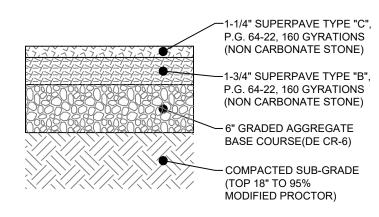
TYPICAL STANDARD PAVEMENT SECTION (TO BE USED WITHIN THE SITE)
