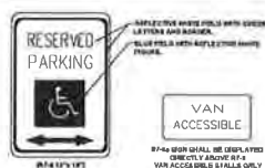
DETAIL: ACCESSIBLE PARKING SIGN (R7-8) SCALE: NOT TO SCALE
