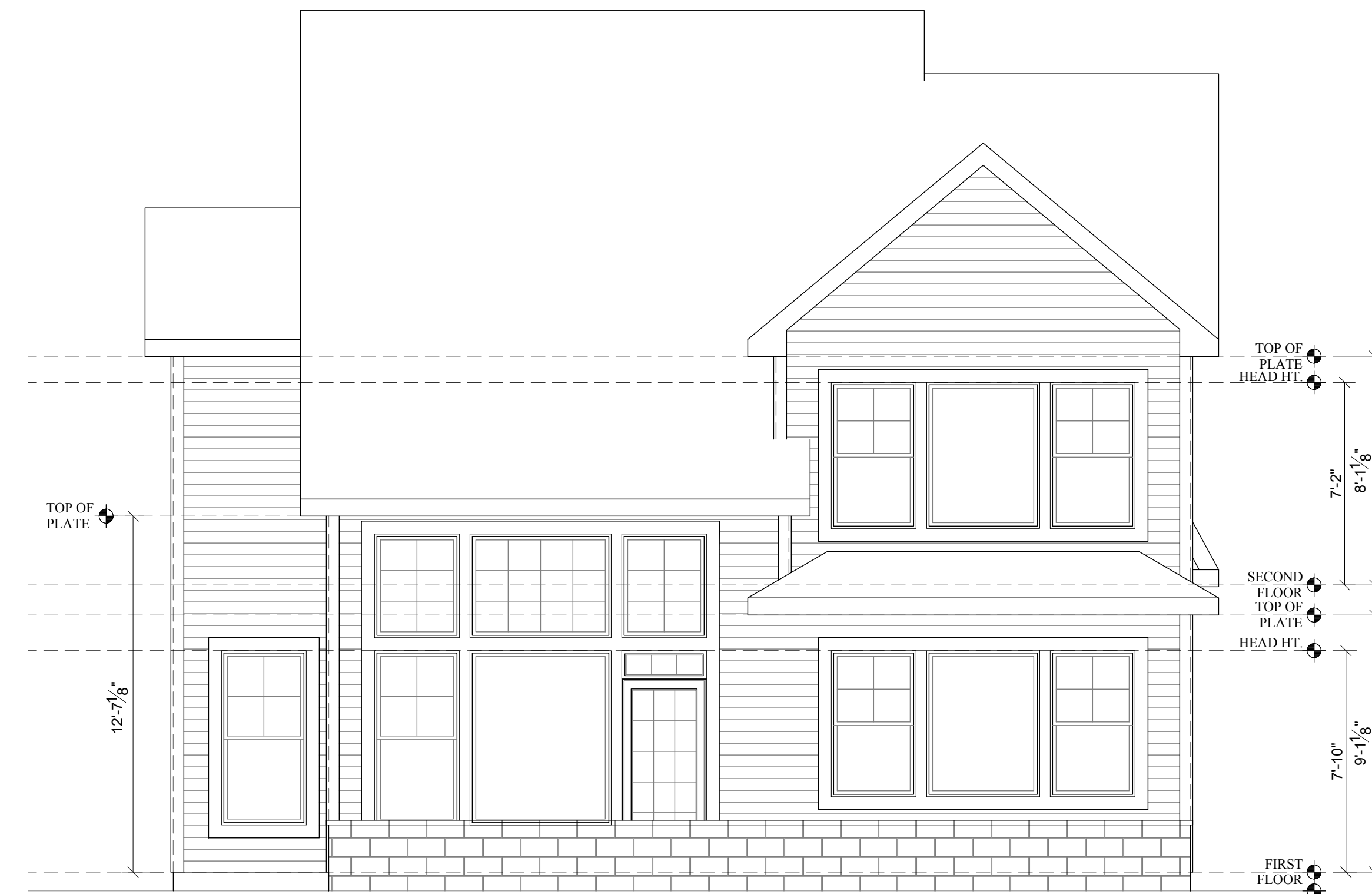
REAR ELEVATION Scale: 1/4" = 1'-0"
