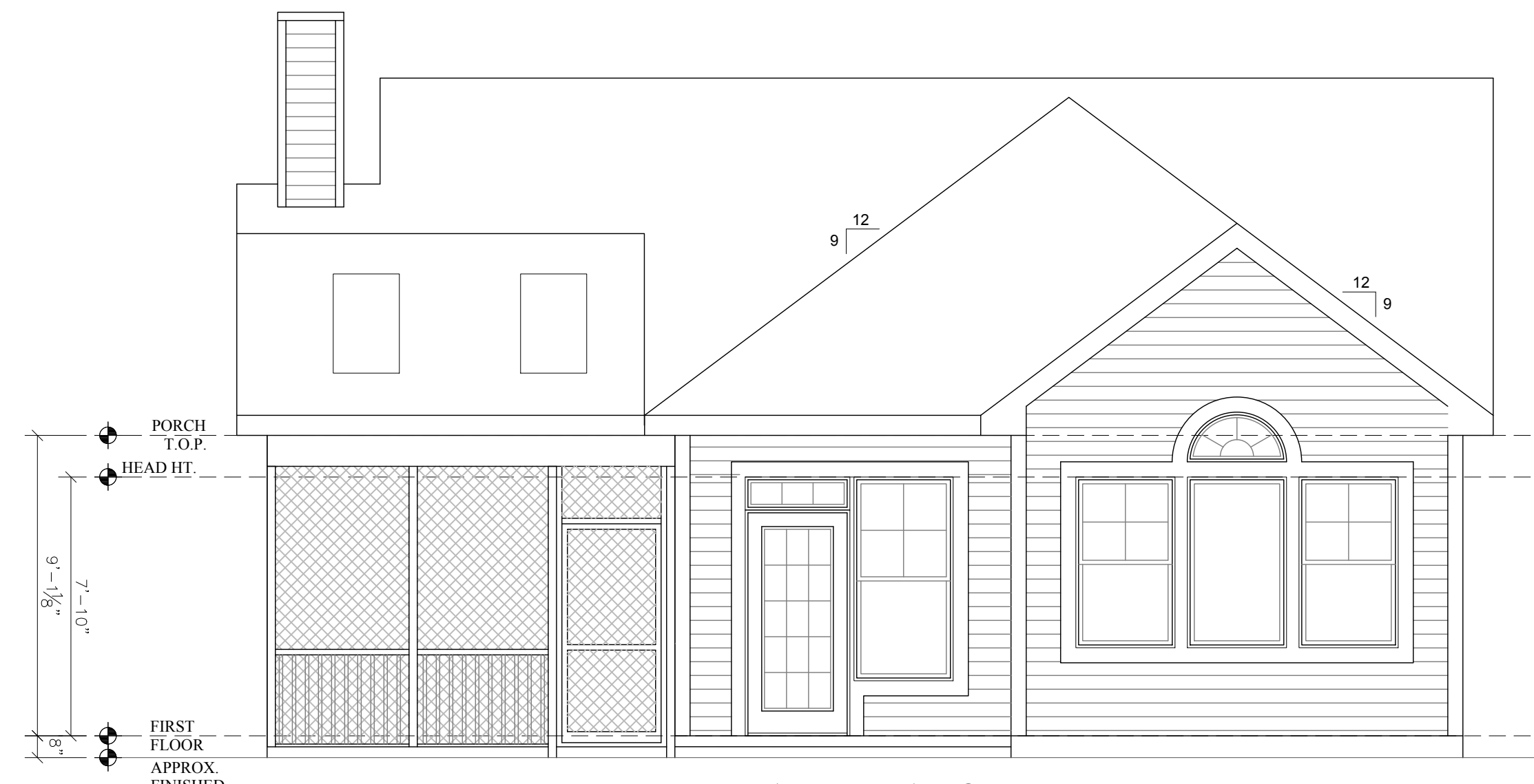
REAR ELEVATION Scale: 1/4" = 1'-0"
