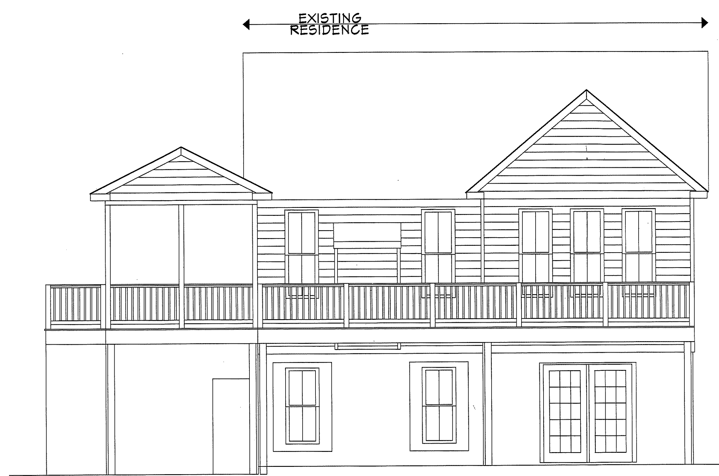
PROPOSED PORCH / DECK ADDITION - REAR YARD ELEVATION SCALE: 1/4" = 1' - 0"
