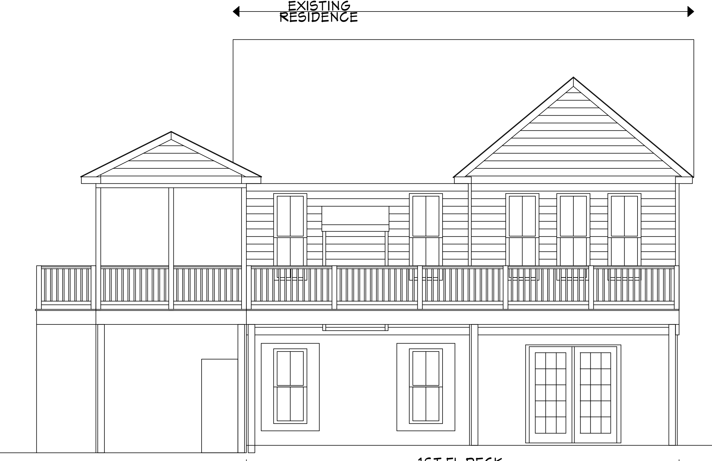
PROPOSED PORCH / DECK ADDITION - REAR YARD ELEVATION SCALE: 1/4" = 1' - 0"
